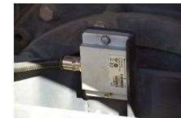
Trimble IC Retrofit Kit: Accelerometer of the CMV system
