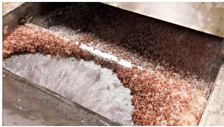
Recycled polymer banknotes in the form of plastic pellets which are then turned into various household products (© CCL Secure).
