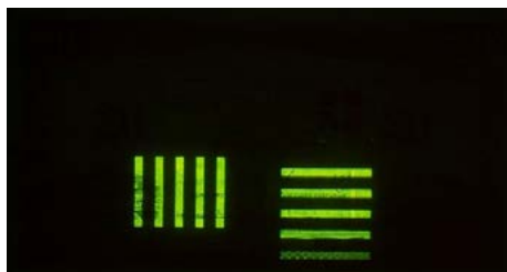
Barcodes on the previous Bank of Scotland £20 paper banknote viewed in UV light.
