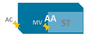
In the image above, we can see that the substation is completely inside the available area AA. Its MV switchgear point is thus also situated inside AA. In this case, the MV placemark is both the MV switchgear and the MV delivery point at the same time.
