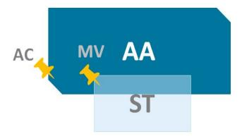
In the image above, we can see that the substation is partially inside the available area AA. Its MV switchgear point is also situated inside AA. In this case, the MV placemark is both the MV switchgear and the MV delivery point at the same time.
