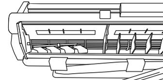
2b. For systems with non-removable drain pan, remove louvers and baffles to access the area behind.
