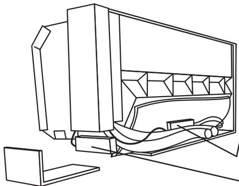
4. Tuck the power supply into the line chase on the back of the ac unit or place it in or under the control box or other secure location.
