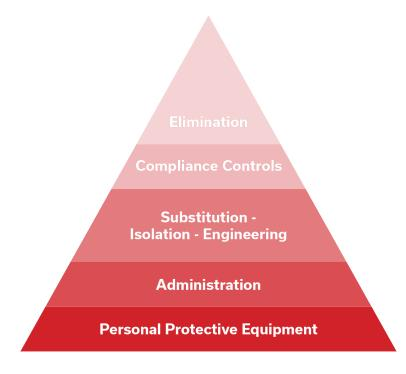
The 5 tiers in the Hierarchy of Control are based on where the control measure is applied – at the source, path, or exposure point of a hazard.
