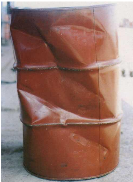
Deep dents. NOT ACCEPTABLE
