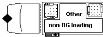
Figure 5.3.6(g): Small vehicle transporting 2 IBCs of same dangerous goods with other non dangerous goods.
