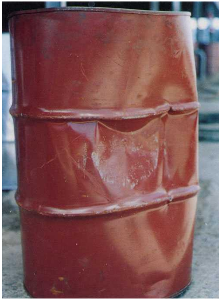
A large dent. NOT ACCEPTABLE
