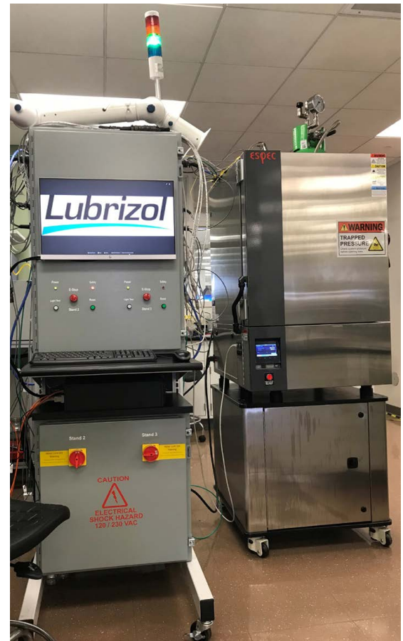
The new ViscoPro 2100 viscometers are enclosed in a mobile benchtop temperature cycling chamber.
