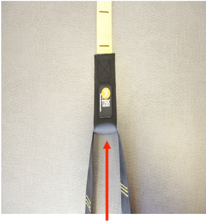
Recalled - no nylon locking loop.
