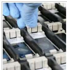
Placement of slides on eXACT™ temperature controlled blocks
