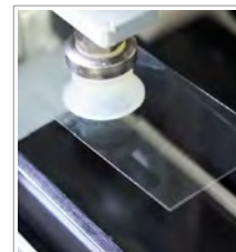
Automated mounting and final coverslip after DAPI
