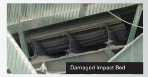
Due to the structure, there was not enough room for two impact beds to be installed at the load zone, so Flexco engineers created Heavy Duty CoreTech Impact rollers which were able to take on the impact outside the impact beds reach.
