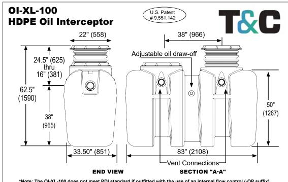
\*Note: The OI-XL-100 does not meet PDI standard if outfitted with the use of an internal flow control (-OP suffix). The PDI standard is only valid with the use of an external flow control fitting.
