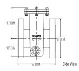
Pressure rating: 150F: 250 Psi / 300F: 400 Psi | PN 10/ PN 16: 16 bar (232 Psi) / PN 25: 25 bar (363 Psi) | Max temperature: 180 °F (82 °C)
