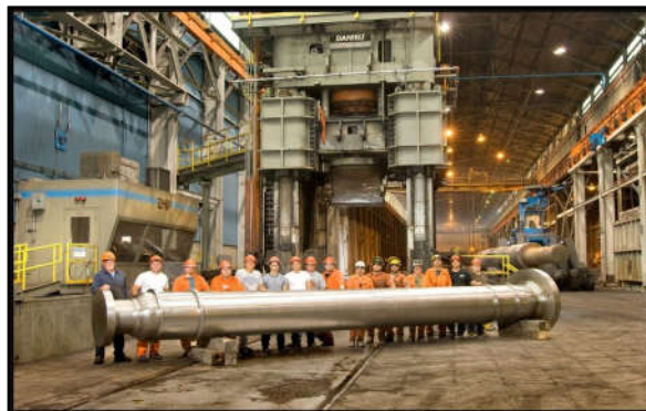
Mine Hoist Shaft
