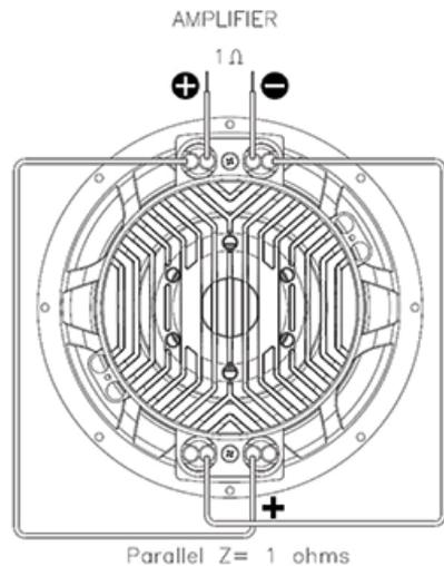
REVO XXX Subwoofers are available in Dual 2 Ohm Impedance only. This means that each subwoofer can be wired for a total impedance of either 4 Ohm (with the 2 voice coils wired in series) or 1 Ohm (with the 2 voice coils wired in parallel).
