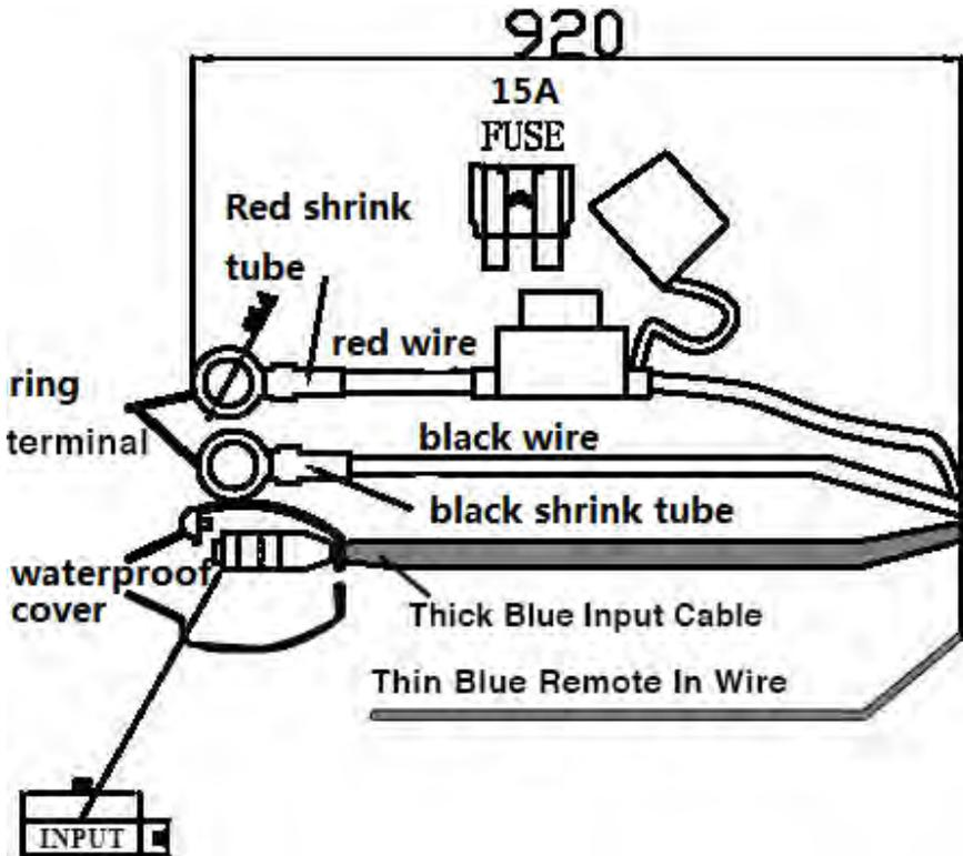
Wet Sounds STEALTH SURGE Soundbars use an operating voltage of 12 volts
