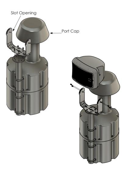
**Step 5** - Position speaker in the bracket so that the threaded holes align with the mounting slots. Thread hardware through bracket into speaker (see Fig A) and position tilt angle of speaker. When the desired angle is set; tighten hardware.
