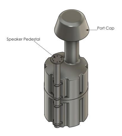
**Step 4** - If using with VS-69 Pro Landscape speakers, mount the speaker bracket to the pedestal using hardware provided with VS-69 Pro. Ensure the bracket slot openings face toward the port cap.
