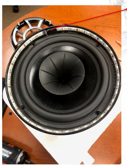
LED STRIP INSTALLED, NOTE RGB WIRE ROUTING. MAKE SURE LED STRIP IS EVENLY PLACED AND IS AGAINST THE DRIVER.
