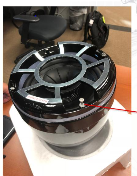
RE-INSTALL GRILL USING THE NEW LONGER PROVIDED SCREWS IN THE RGB LED RING KIT.
