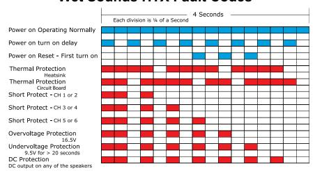
For HTX 4, 6 amplifiers, a short will only shut down the channels which are in fault. The other channels will continue to play. After a fault connection is cleared, the error code will continue to flash, while the logo is still illuminated blue. Please contact Tech Support for additional assistance, questions, etc.
