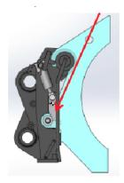
V-Loc Coupler wedge locks the attachment tight to the stop even when pins are
