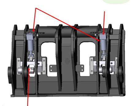
Dual Cylinder Design with P.O. Check Valves ensure cylinders will not retract if hydraulic hoses are damaged
