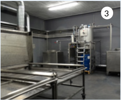
1: Cleaning of hoses 2: Racks for ink trays and doctor blades, 3. Distillation systems and integration between parts washer, tanks, and distiller.
