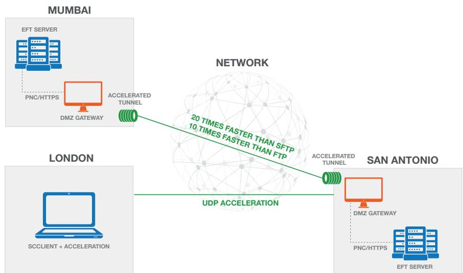
The Accelerate module is configured and managed in the EFT administration interface as part of an integrated system. The FAST protocol can be used in Copy/Move Actions and Download Actions in EFT Event Rules to automatically copy, move, and download files, and with scClient from the users' desktops.
