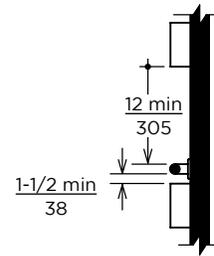
**Fig. 17f Protruding Objects Mounted near Grab Bars.**
