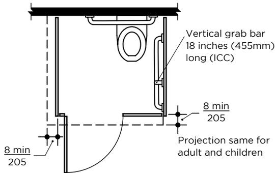
**Fig. 15b Horizontal Toe Clearance. (2017 ICC Standards)**
