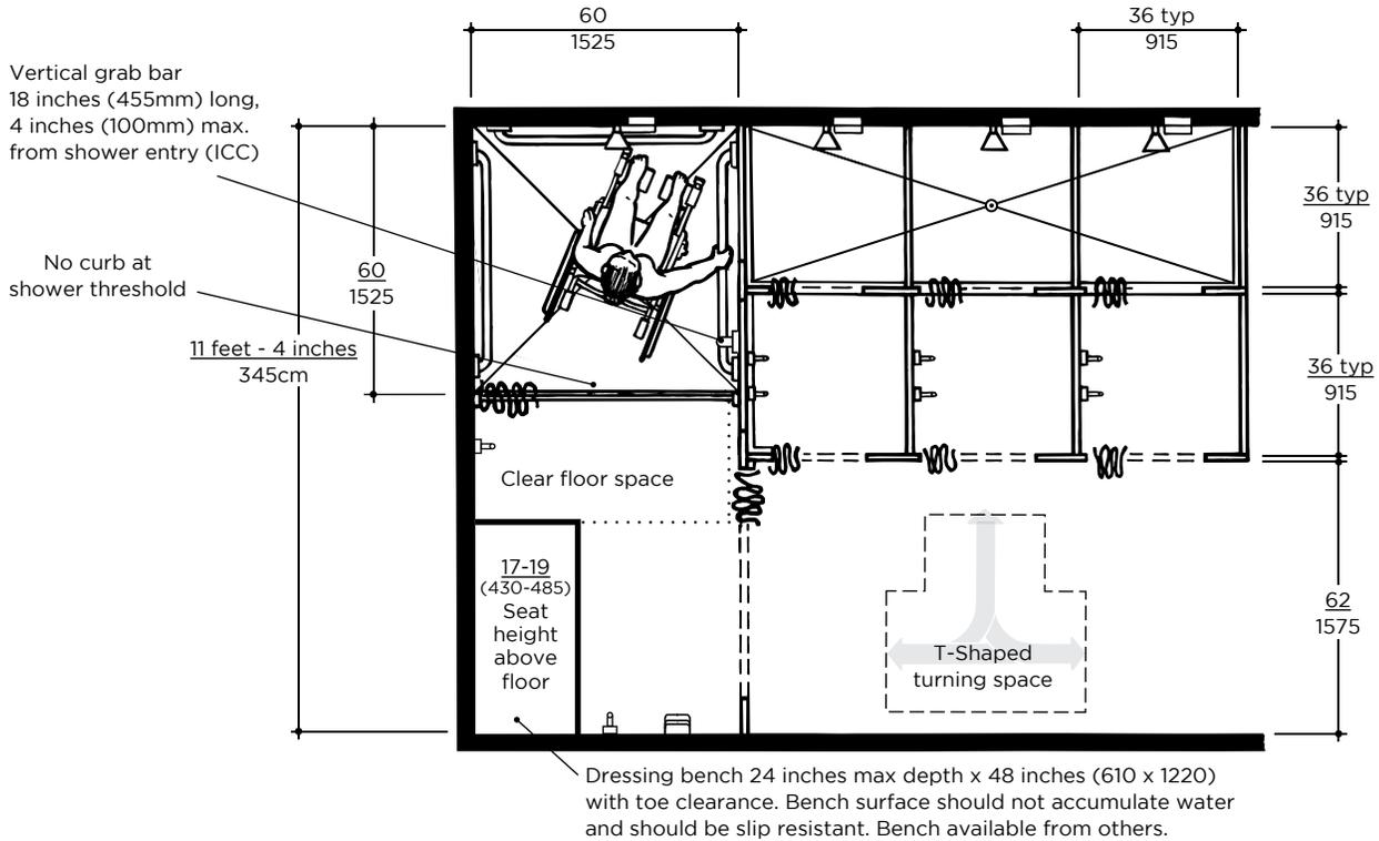
**Fig. 42 Multiple Shower Installation with Transfer Shower Compartment and Dressing Compartment.**
