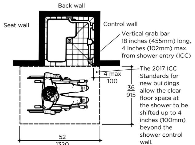
**Fig. 28c Required Clear Floor Space. 2017 ICC New Buildings**
