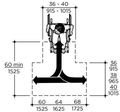
**Fig.5b T-Shaped Turning Space 2017 ICC Standards**
