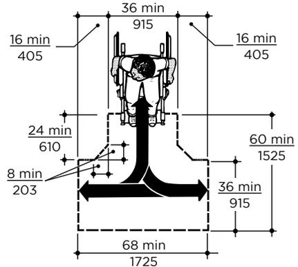
**Fig.5c T-Shaped Turning Space. 2017 ICC New Buildings**
