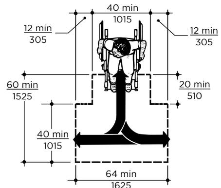
**Fig.5e T-Shaped Turning Space. 2017 ICC New Buildings**
