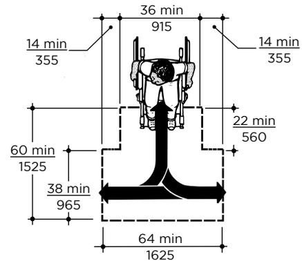
**Fig.5d T-Shaped Turning Space. 2017 ICC New Buildings**
