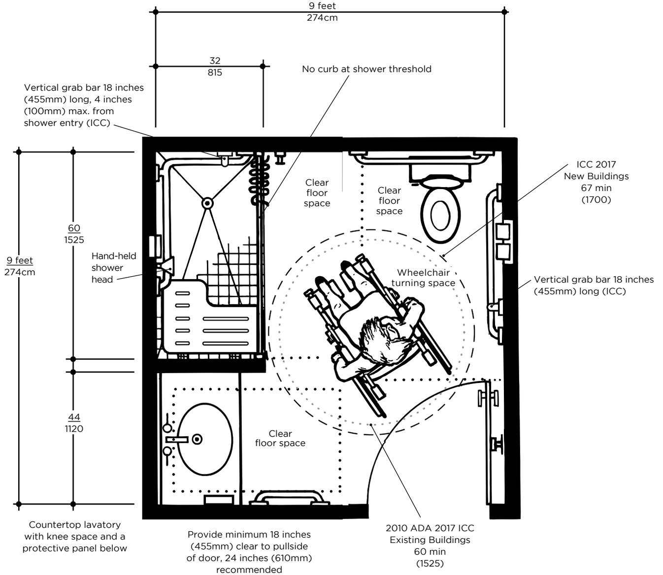
**Fig. 38 Bathroom with Enlarged Alternate Roll-in Shower Compartment.**
