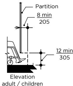
**Fig. 15d Vertical Toe Clearance. (2017 ICC Standards)**
