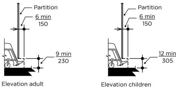
**Fig. 15c Vertical Toe Clearance. (2010 ADA Standards)**
