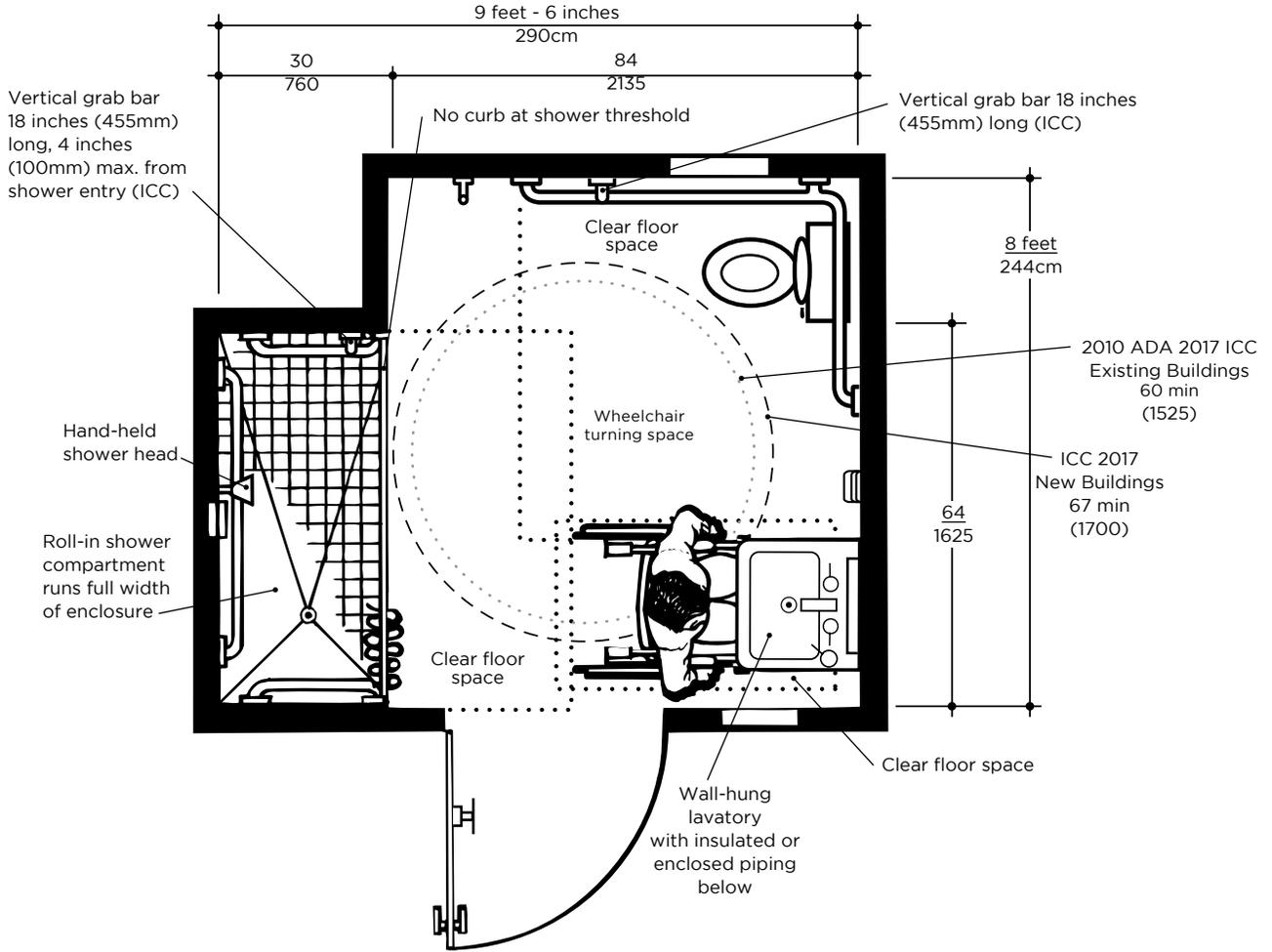
**Fig. 36 Bathroom with Enlarged Roll-in Shower Compartment.**
