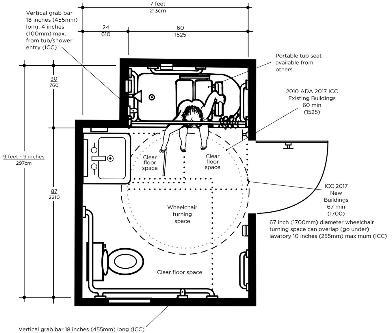
**Fig. 40 Bathroom with Combination Tub/Shower Unit with Permanent Seat.**
