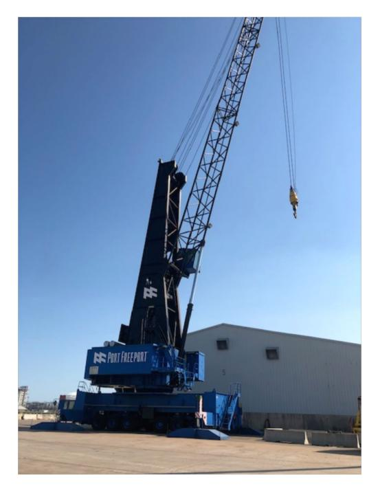
GOTTWALD MOBILE HARBOR CRANE MODEL HMK 280 E (Year 1997) SERIAL NUMBER: 128278 LOCATION: PORT FREEPORT TEXAS (one owner) OPERATING HOURS: 17879 (very low for a 1997 crane) CONDITION: Good working condition with regular maintenance performed. Crane runs smoothly and is used regularly in cargo and container handling operations. Always maintained ready to work. IMPROVEMENTS: Diesel engine replaced. Crane control system upgraded. ADDITIONALS: Includes a spare parts package and 2 x Bromma spreaders
