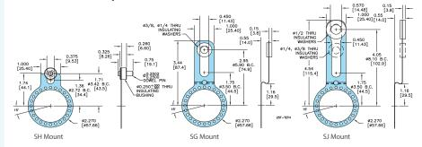
All dimensions are in inches with a tolerance of +0.005" or +0.01" unless otherwise specified. Metric dimensions are given in brackets [mm].
