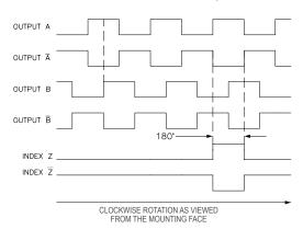
NOTE: ALL DEGREE REFERENCES ARE ELECTRICAL DEGREES. COMPLEMENTARY SIGNALS  $\bar{A},\bar{B},\bar{Z}$  APPLY TO LINE DRIVER (HV & H5) OUTPUTS ONLY.
