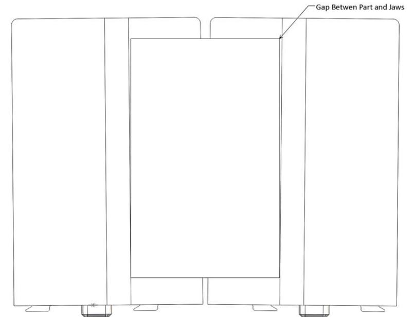
\* This type of jaw deflection does not occur when MultiGrip Jaws are loaded into a MultiGrip Vise
