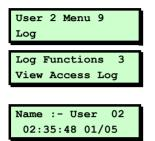
You can use this option to view the content of the access log, which stores every use of a user code of type Access (which is used to open doors).
