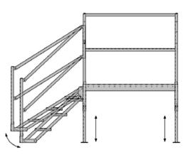
The adjustable legs and pivoting steps make the Omni Step the perfect solution for uneven terrain on any project site.
